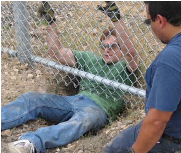
Two men with hand tools can dig under a typical unburied fence in 11.1 minutes.
